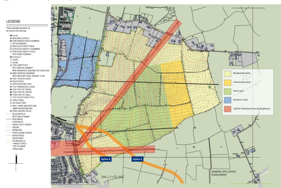
Note, that Plate 1 shows two alignment options for the Mayfield Kilbarry Link Road. Option A is the LAP identified route; this creates a large cut through the hillside. Option B is a route that more naturally follows contours and has less of an impact (less cut).
